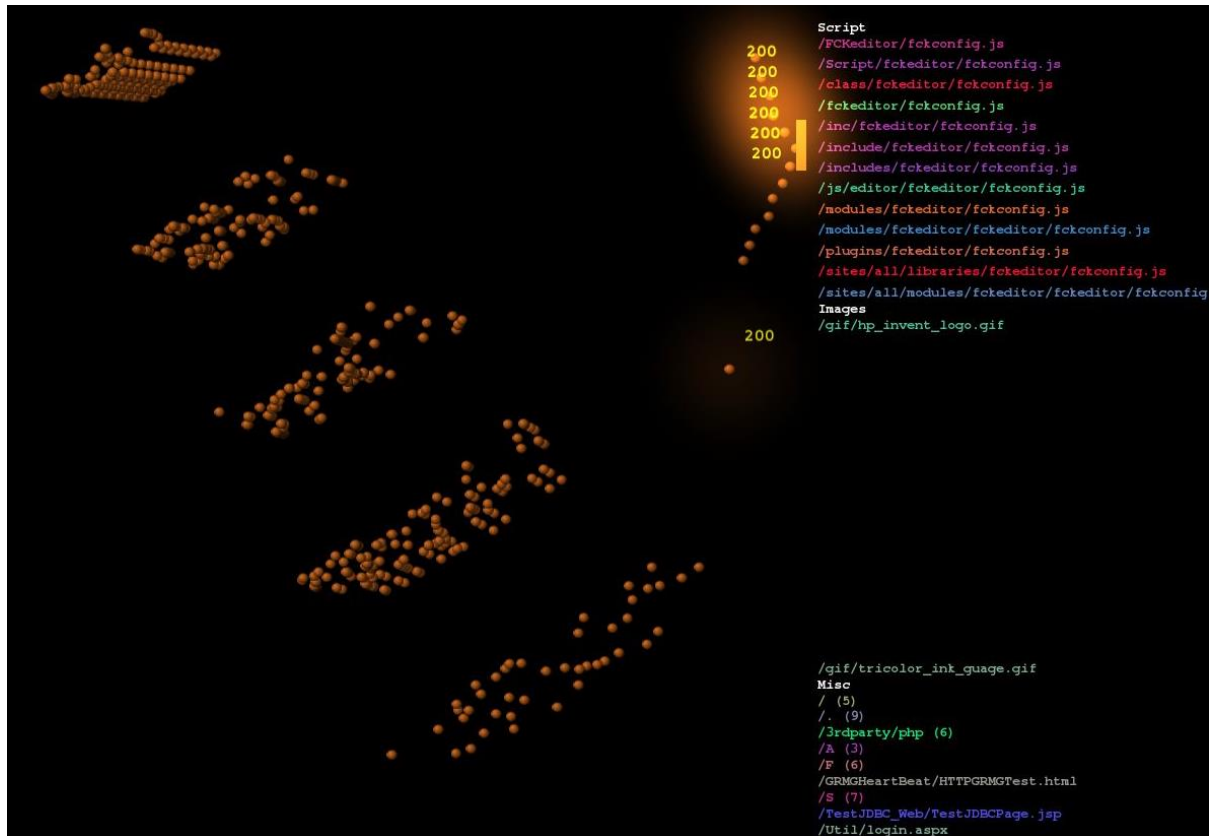
Figure 30. Using Logstalgia to visualise penetration testing with Nikto2 towards the prototype web server.
