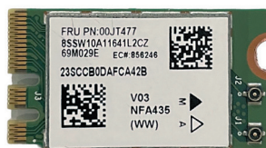
FIGURE 20: QUALCOMM ATHEROS WI-FI M.2 CHIP
